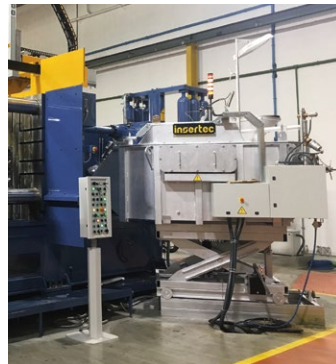
\ DMAE dosing furnace
