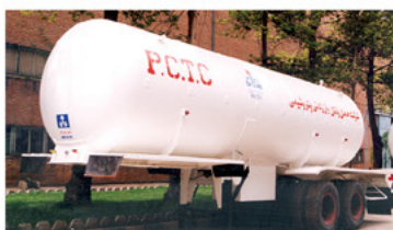
Ammonia Semitrailers Cap. : 29700 L.
