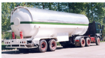
LPG Semitrailers Cap.: 12000 Gal.
