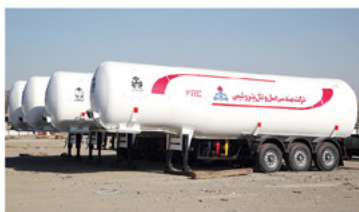
Ammonia Semitrailers Swan Shape Cap: 11700 Gal
