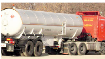
Propane Semitrailers Cap. : 9800 Gal.
