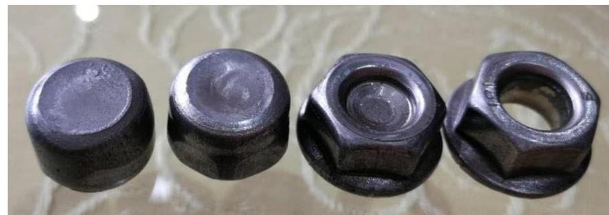
$R_m = 519\text{MPa}$ ,  $Z = 59\%$ ,  $HRB = 75$ , 1/3冷顶锻合格
